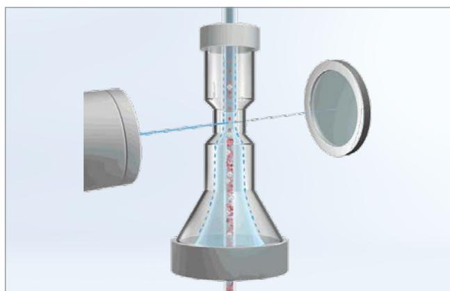
**Fig. 4** Hydrodynamic focusing of urine particles inside the flow cell of the UF-series instruments
