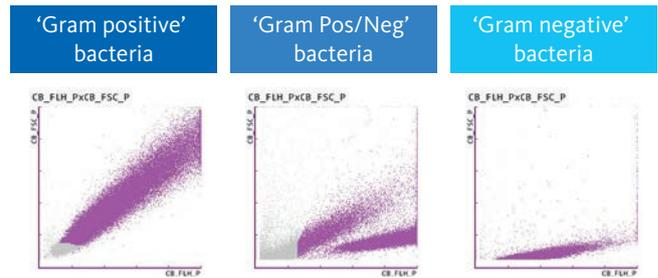
**Fig. 7** Detection of Gram-positive and Gram-negative bacteria by fluorescence flow cytometry on the UF-5000
