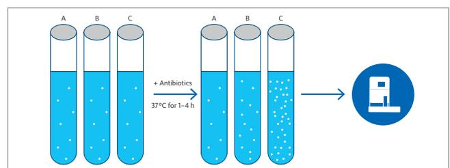
**Fig. 11** Alternative antibiotic susceptibility testing on the UF-5000 via growth monitoring of bacterial isolates in broth supplemented with different antibiotics. The bacteria concentration correlates to (A) highly effective, (B) medium-effective and (C) ineffective antibiotics.
