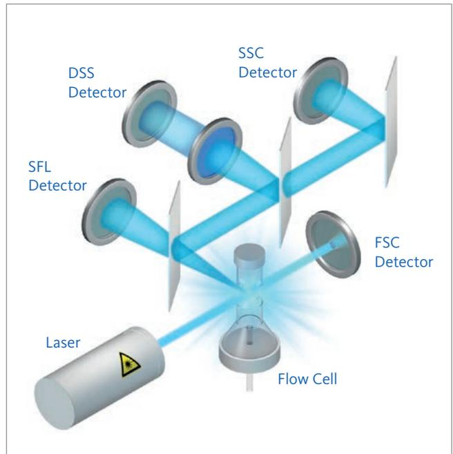
**Fig. 5** Fluorescence flow cytometry on the UF-series. A laser beam is directed at the flow cell, hitting all the particles passing through. Fluorescence light is emitted from excited electrons of the fluorescence dyes and, depending on the individual particle type, the oncoming laser light is characteristically diverted. Photodetectors recognise individual particles, and based on the individual signal patterns, the signals are plotted in a scattergram.
